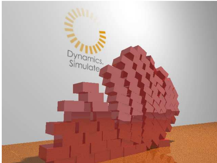
Figure 5: Frame from the simulation of a brick wall. Frictional contact is present between the bricks in the wall and between the bricks and ground.
